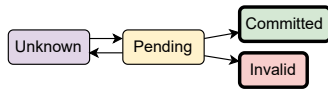
Figure 4: Transaction statuses and transitions. Committed and Invalid states are final, once observed the alternative final status will never be observed (except after disaster recovery).
